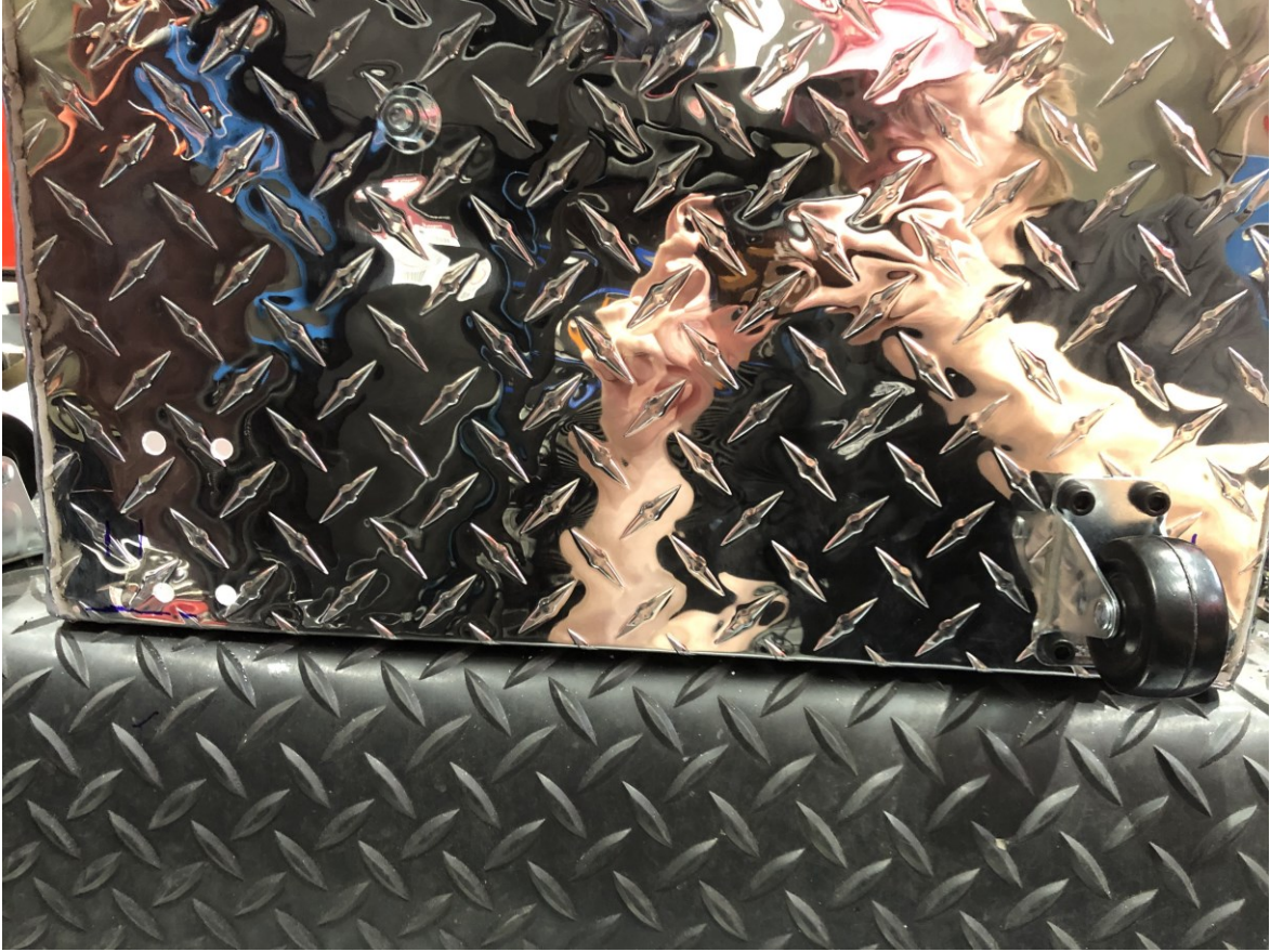
Figure B.29 The casters leveled, aligned, and mounted on the lower left-hand side of the toolbox
