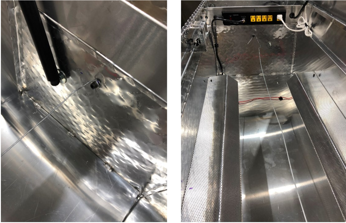
Figure B.27 The aluminum hanging wire mounted in the toolbox by the 1/4" bolts in each end
