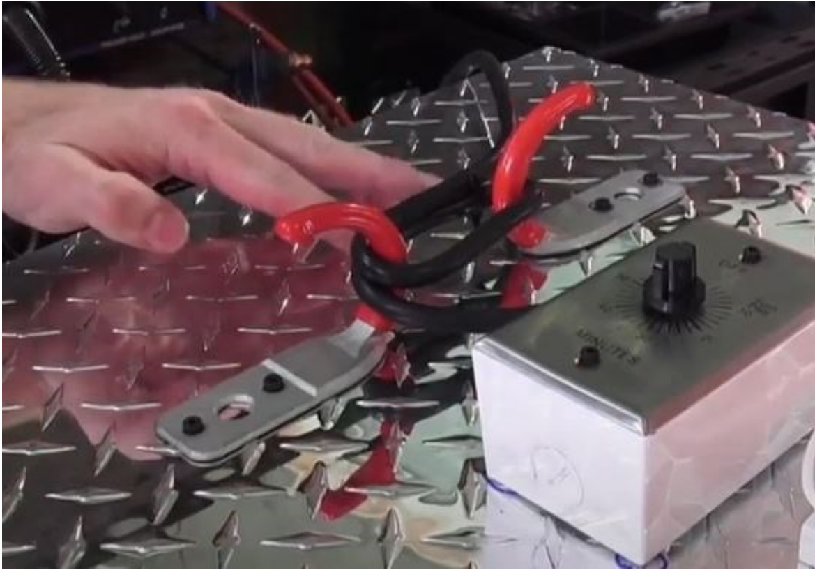
Figure B.18 The strain relief of the power cable on the J-hooks with zip-ties
