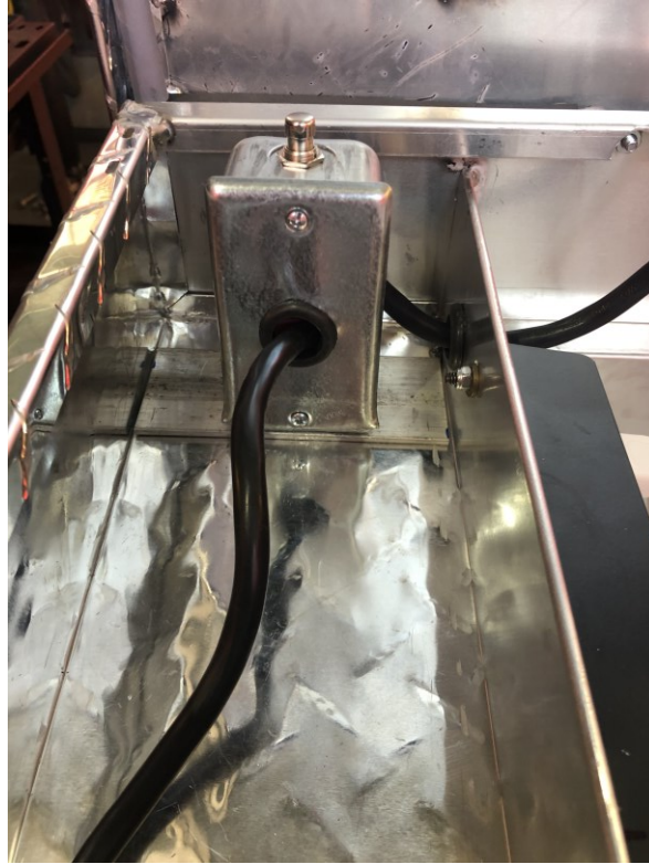
Figure B.21 The RACO internal switch box cover shown mounted to the RACO internal switch box
