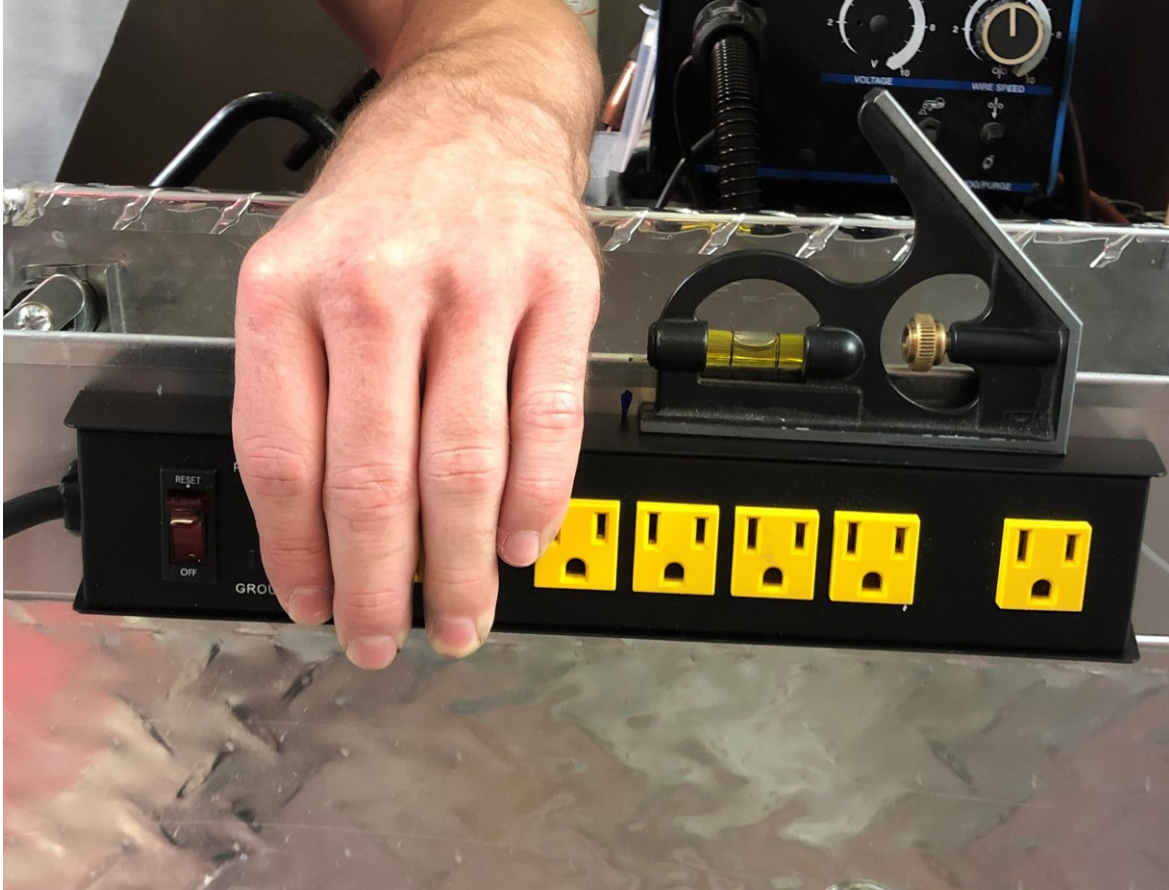
Figure B.7 The leveled power strip with the power cord facing the front of the toolbox
