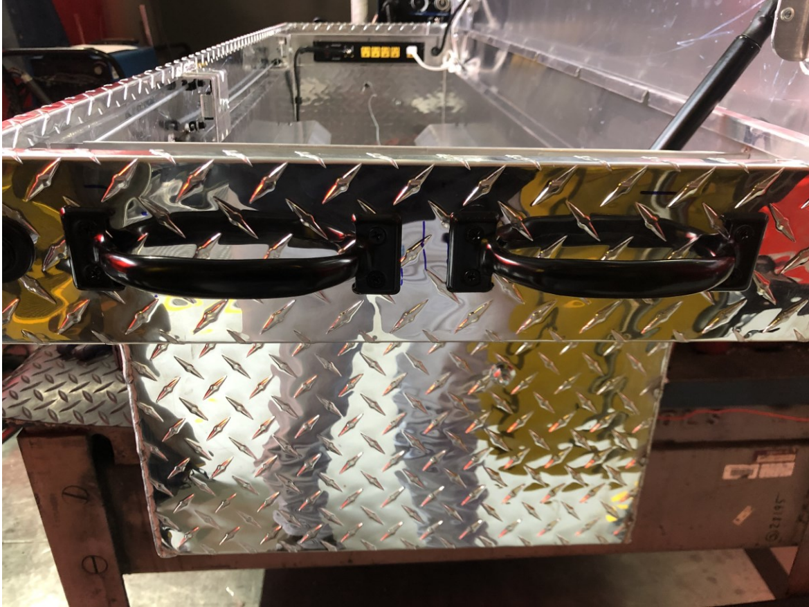
Figure B.28 The tow handles leveled, spaced, and mounted onto the upper right-hand side of the toolbox
