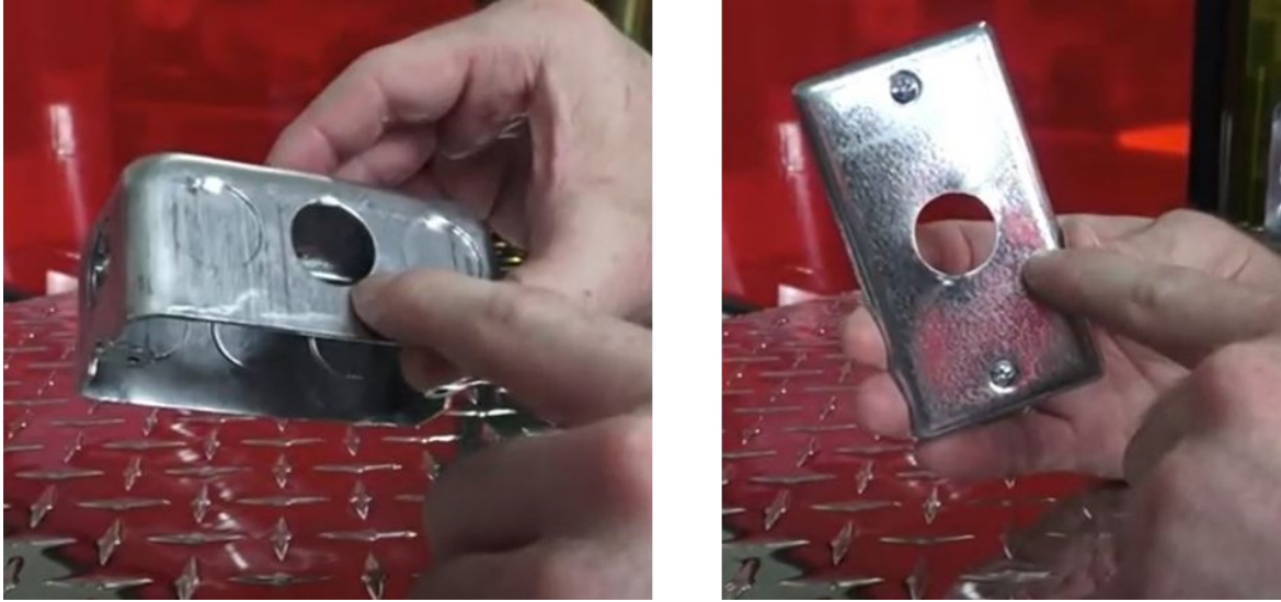
Figure B.10 The side and front cover punched out holes in the RACO internal switch box and cover
