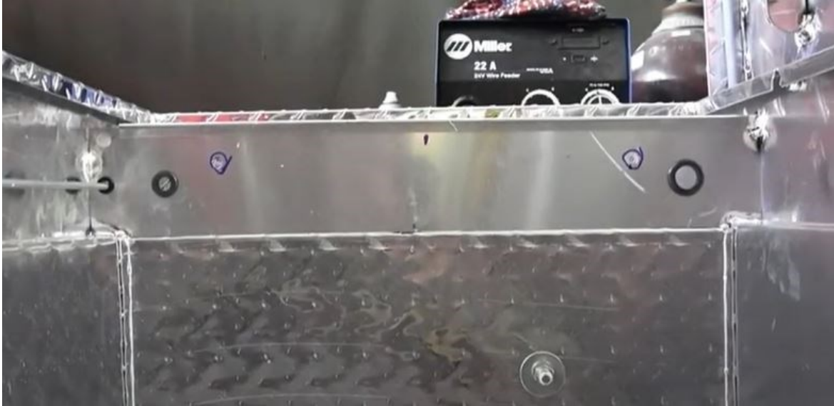
Figure B.6 The four mount holes drilled in the upper left-hand plate in the inside of the toolbox
